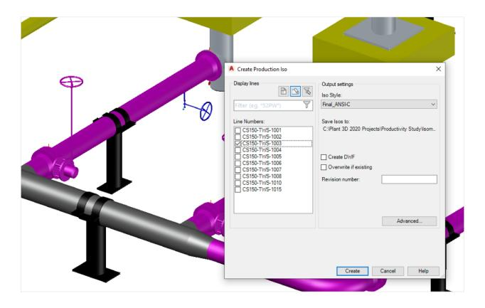
After selecting the type of isometric and the line(s) to be created, the drawing process takes place as a background task, allowing the user to continue with other work. The Plant 3D toolset notifies the user when the creation process has been completed and when the drawing is **ready to be opened:**
