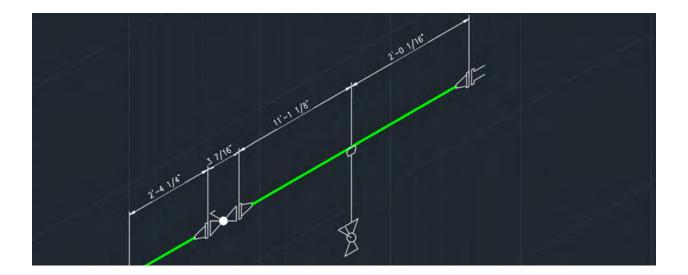
Since the isometric drawing is not to scale, all the dimensions need to be entered. Also, the MTO table must be entered manually as an AutoCAD table, thus requiring a lot of input even for an experienced AutoCAD user.
