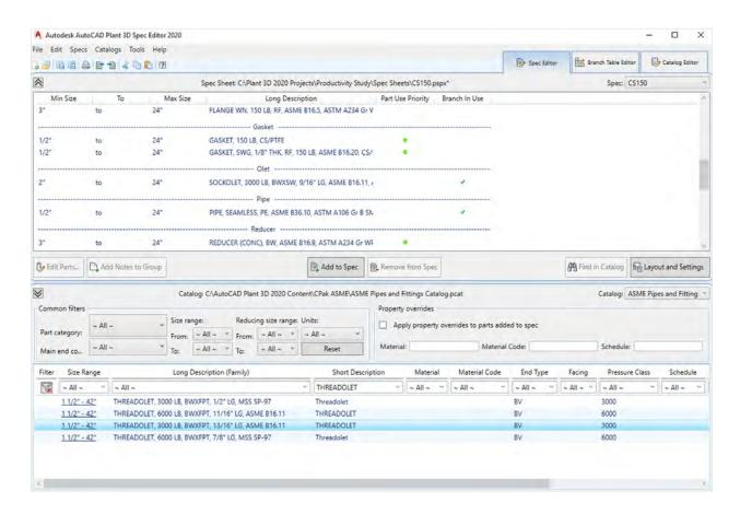
Using the 'Add to Spec' command automatically adds the selected threadolets to the pipe spec. The Plug and nipples are added in the same way.
