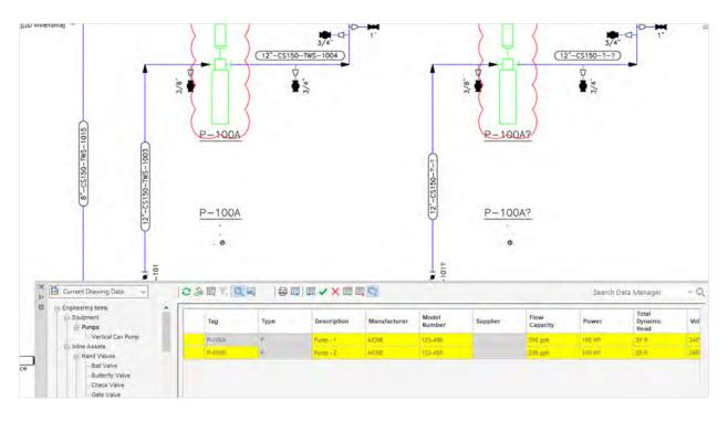
Using the Report Creator, designers can generate the equipment list directly from the P&ID database, avoiding errors or omissions. There is no direct comparison with basic AutoCAD, unless some customized script is written to extract property data from blocks.
