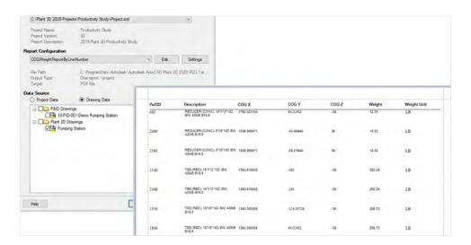
Using basic AutoCAD, this task is usually performed using an Excel spreadsheet. It's a manual task, and designers must check to ensure no items are missing. Also, there is no link between the spreadsheet and the data source, so changes made in basic AutoCAD require a manual update of the spreadsheet.
