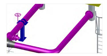
The designer then inserts the valve by selecting it from the spec and identifying the insertion point in the pipe.
