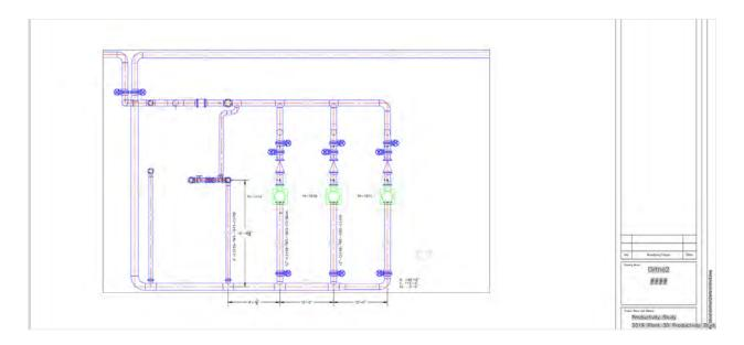
After creating the viewport, the designer can use the Plant 3D toolset 'annotation' commands to add equipment tags, line numbers, piping elevations, etc. The toolset employs standard dimensioning to place linear dimensioning:
