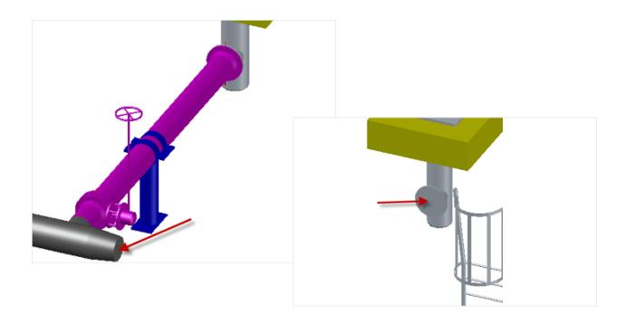
The designer simply selects the 'route pipe' command and selects the pipe route. In this case, the end of the pipe at the reducer and the pump nozzle:
