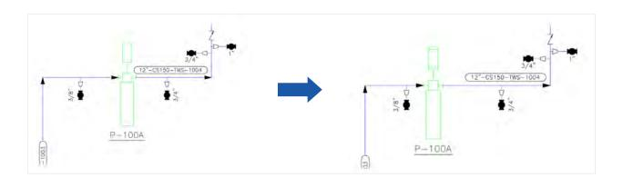
The second task is to add instrumentation. The process is very similar when using basic AutoCAD, except that with the toolset, connectivity is understood while connecting instruments:
