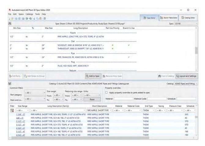
Once the piping spec is saved, the updated spec is available for use in the Plant 3D toolset modeler.
